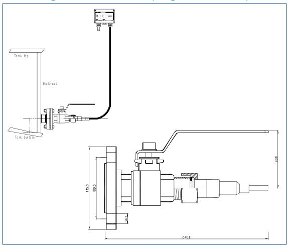
Flange, valve and nut are manufactured of ASTM 316L steel. The gaskets are made of nitrile rubber.
